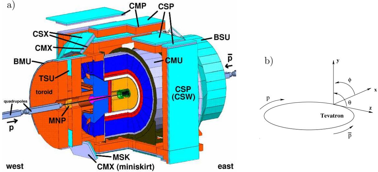
Abbildung 2: a) Isometric view of the CDF detector in Run II with the abbreviations of the different components of the muon system. The inner green and orange part represents the tracking system and the blue one the calorimeters. b) The coordinate system of the CDF II detector.
