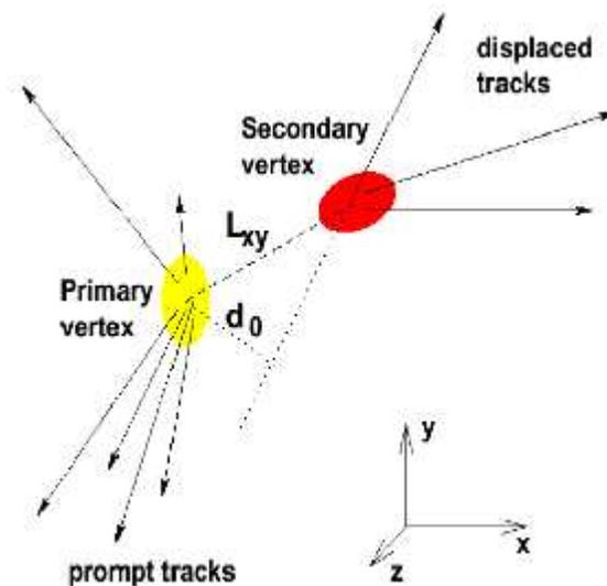
Abbildung 8: General principle of  $b$ -tagging. The impact parameter  $d_0$  and the decay length  $L_{xy}$  are sketched.
