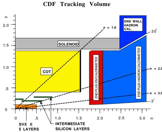
Abbildung 3: Longitudinal view of the CDF tracking system.
