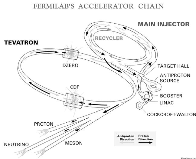
Abbildung 1: *Schematic overview of the TEVATRON accelerator with its two detectors D0 and CDF and its preaccelerators.*
